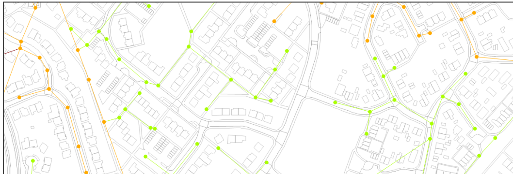
Figure 1 – A small area within a typical 1D network showing manholes and conduits
