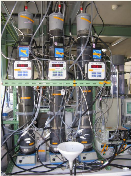
3 lab scale PROVEO digesters (10 L)
